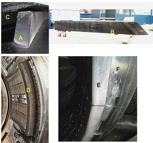
Fig. 2. Location of the analyzed DCL: neutralizers (A: leading edge, B: lateral tiles), C: underside of the TPL fingers, D: lateral faces of C2-launcher and outboard modular limiter (E: CFC and F: copper).
